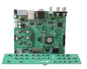
NVP1918C includes 8-Ch 960H video decoder and 9-Ch audio codec, which guarantees high quality images. It accepts separate 8 CVBS inputs from camera, TV, DVD and the other video signal sources. It digitizes and decodes NTSC/PAL/COMET video signal into digital video signal which represents 8-bit ITU-R BT.656/1302 4:2:2 format with 27/36/54/72/108/144MHz multiplexed. Each video output can be selected between 720H and 960H. 9-Ch audio codec is 8-Ch PCM
