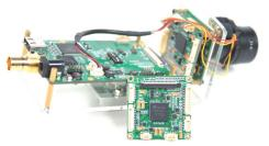
The brand new megapixel CMOS ISP, NVP2410, with state-of-the-art imaging technology, will bring you a whole new world of image quality. It is designed for Full-HD quality surveillance cameras like HD-SDI(HDCCTV) and Full-HD IP cameras as well as highend analog cameras. It supports up to 60 fps Full-HD(1920×1080) input and output, second to none technology in video surveillance industry. For further process, it receives
