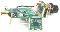
The brand new megapixel CMOS ISP, NVP2420/NVP2421 has state-ofthe-art technology to give the best image quality ever. It is designed for Full-HD surveillance cameras like HD-SDI(HDCCTV), Full-HD IP camera and high-end analog camera. It can support up to 1920 X 1080 @ 60 fps input and output. It receives 12-bits parallel or various sub-LVDS CMOS sensor inputs. Output is provided as BT.656, BT.1120, YC 16bits and composite
