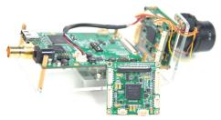
The brand new megapixel CMOS ISP, NVP2423 has state-of-the-art technology to give the best image quality ever. It is designed for HD surveillance cameras like HD-SDI(HDCCTV) and Analog HD camera. It can support to 1.3M CMOS sensor input and output I/F as digital(720p) and analog 960H(CVBS). It receives 4 channel sub-LVDS CMOS sensor inputs. NVP2423 includes groundbreaking functions, for example, N-WDR(Natural
